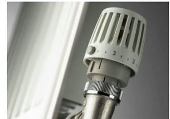
What the 1 to 5 or 6 settings relate to is the air temperature at which the radiator will be turned off. A 1 to 5 thermostatic radiator valve at setting 5 makes the radiator turn off when the adjacent air temperature is roughly 25°C, and at setting 1 it will turn the radiator off at around 15°C. Thermostatic radiator valves can be retrofitted and are relatively cheap to install. Make sure to leave the space around the valve clear for it to be able to measure temperature properly.
